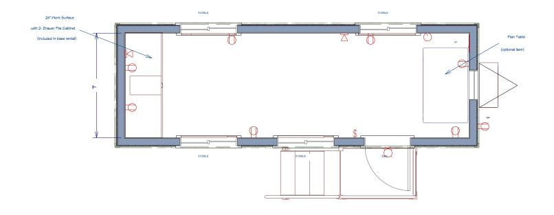
LEGEND E Panel Box Porch Light Thermostat Duplex Outlet SLight Switch KEmpty data box me Perm. Interior wall me Temp. Interior wall
